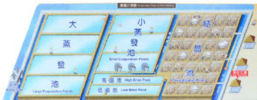
Fig.7 The process of Tile-paved salt field
